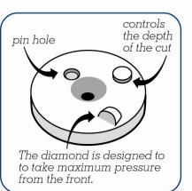
Two configurations can be used for the STI Wolverine PCD Cutters. One is more aggressive than the other. It is very important that installation is followed according to these instructions. Improper installation will result in premature wear of the diamonds and possible breakage. STI is not responsible for diamond breakage due to improper installation and/or rotation.
